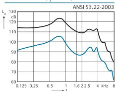
Frequency Response ( $L_i = 60 \text{ dB}$ ) **Basic Frequency Response** ( $L_i = 60 \text{ dB}$ )
